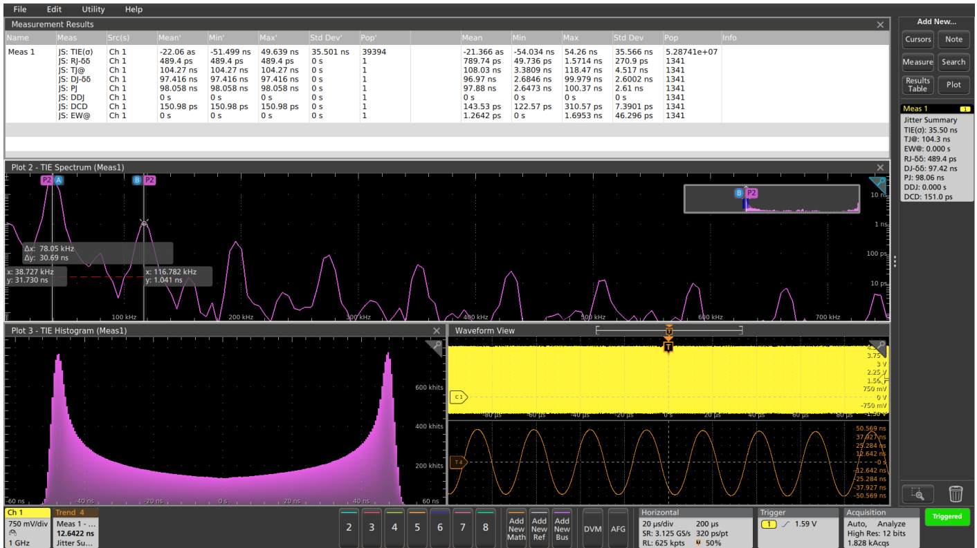
FIGURE 7. The 5 Series MSO Jitter Summary characterization of a 98 MHz spread spectrum clock.
