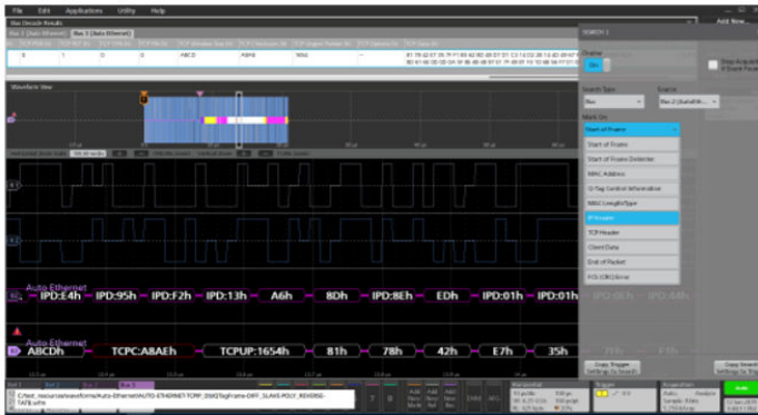
100BASE-T1 Protocol decode solution
